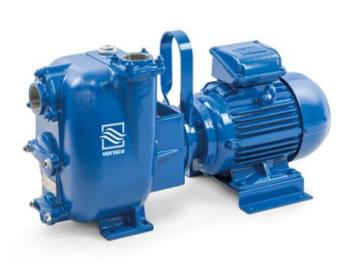
Product Data Suction port Threaded - 2" ISO 228 (BSP) Delivery port Threaded - 2" ISO 228 (BSP) Qmax 50 m<sup>3</sup>/h - 833 I/min (220 USgpm) Hmax 53 m (174 ft) Solids handling 13 mm (0.5 ") Motor power 7,5 kW - 10 HP
